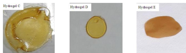
Fig.1: Hydrogel C (Psyllium-PVA-Casein-hydrolysate-PAA-agarose-PEG) with 20% polyacrylamide & 0.7% agarose. Hydrogel D (Psyllium-PVA-Casein hydrolysate-PAA-AG-PEG) with 20% polyacrylamide), Hydrogel E (Psyllium-PVA-CH-PAA-AG-PEG) with 1% agarose
